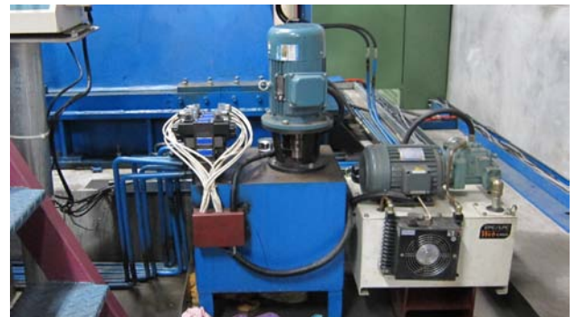
Hydraulic Actuator AO-P is used on a Steel Web Finishing Machine for Rewinding
